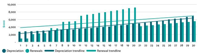
In preparing the renewals profile for stormwater, a range of technical information and asset life data has been considered. These detailed assumptions and parameters are contained within the AMP. Broadly speaking, renewal requirements are based on Council's Asset Survival Model, which uses historical CCTV information to estimate the proportion of assets that survive to a given age (and, by extension, the proportion of assets that will fail at a given age).
