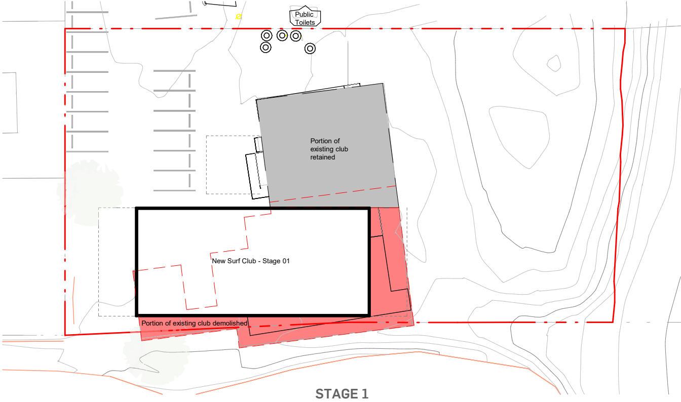
STAGE 1 - Kitchen and Lounge retained - Storage, Change, WC's, Tower need to be accommodated elsewhere during Stage 1 construction
