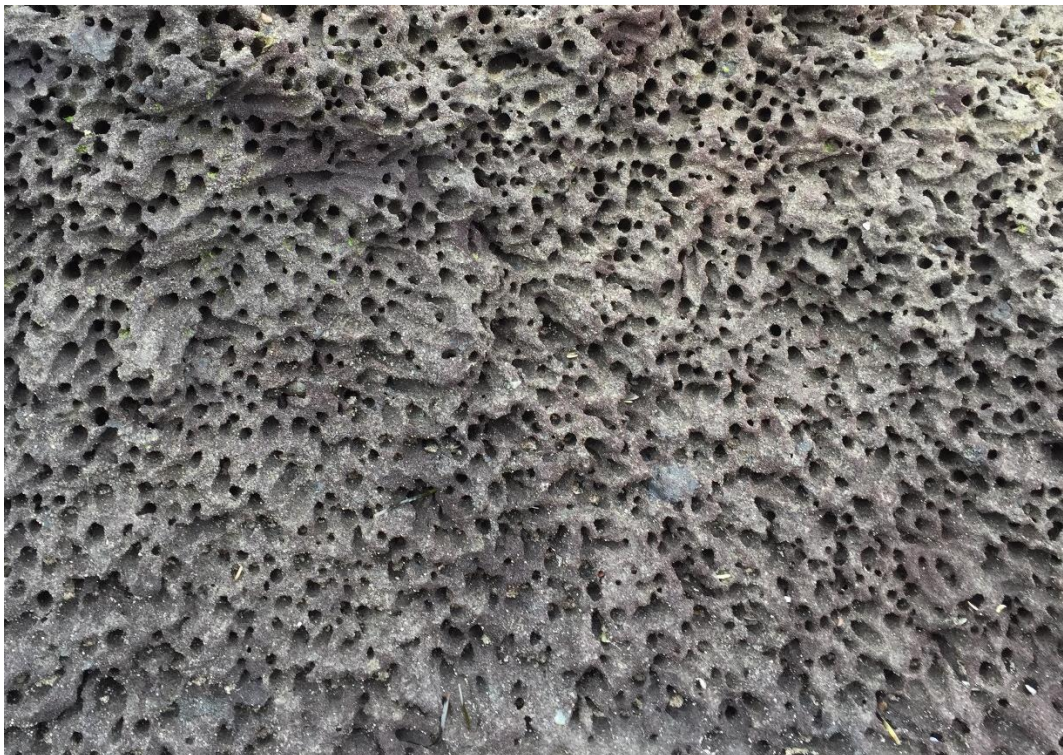
Figure 10: Intense surficial boring of extremely weak rock exposed within the intertidal zone
