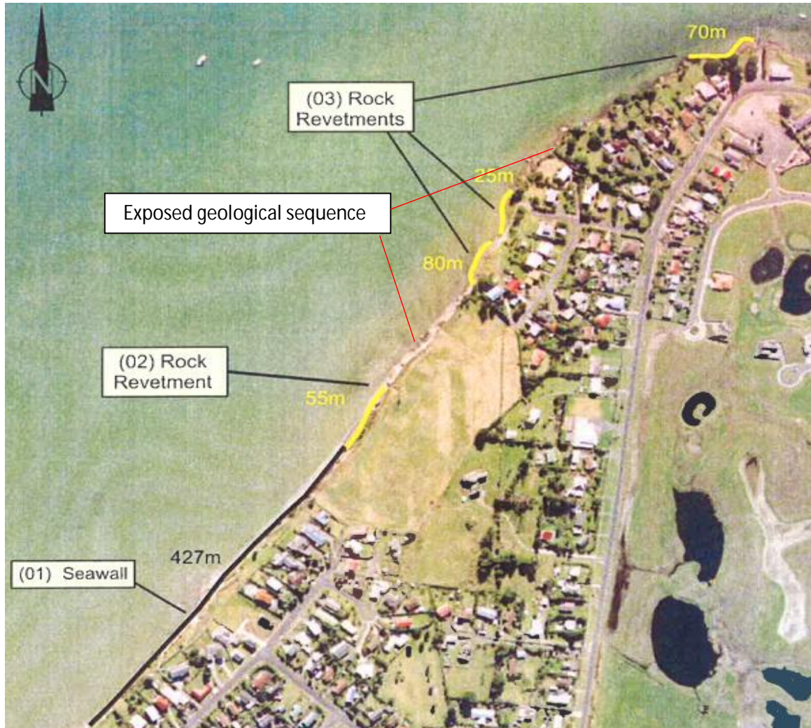
Figure 2.2 Coastal protection works and location of exposed geological sequence- One Tree Point West Source: NRC 2009 & T+T 2017
