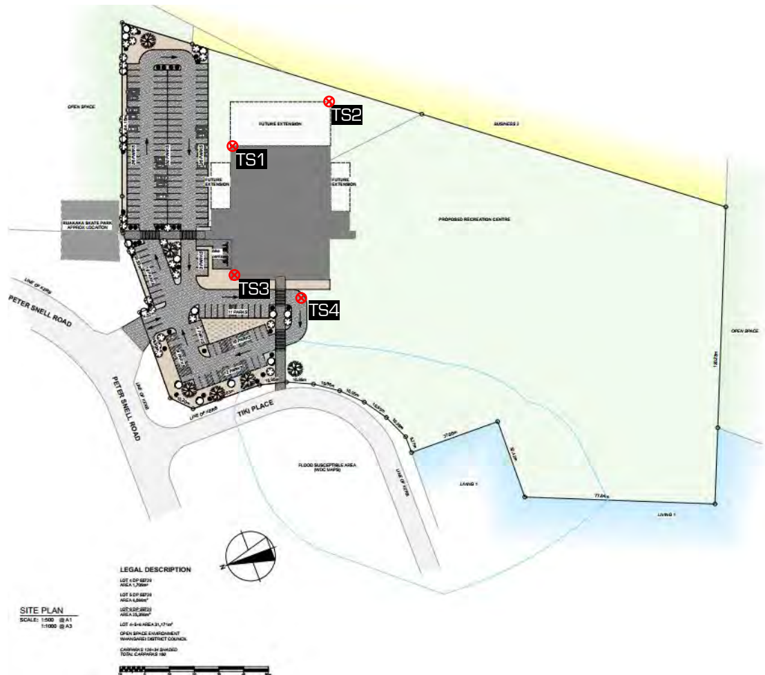
Figure 3: Plan drawing of site showing outlines of the proposed development with borehole (TS) locations. Supplied by HB Architecture.
